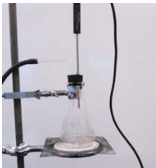
Figure 1 The distillation apparatus fitted with a Vernier temperature probe.
