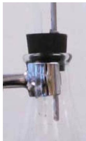
Figure 2 The placement of the temperature probe in the flask.
