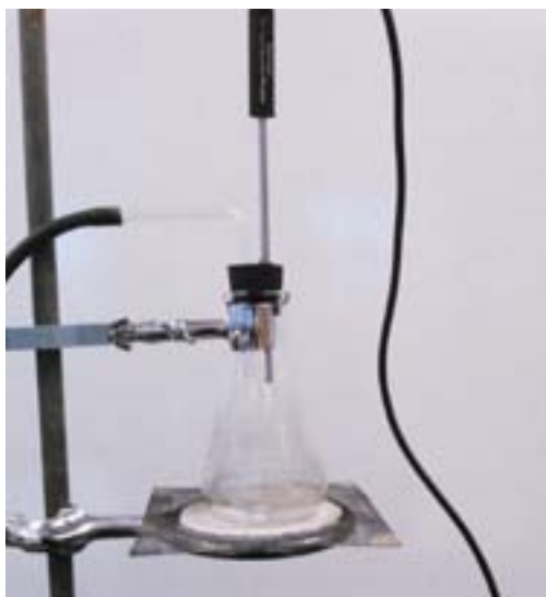
Figure 1 The distillation apparatus fitted with a Vernier temperature probe.
